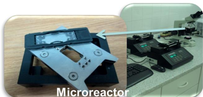
Setup of the commercial microreactor (Micronit Microfluidics BV) system
