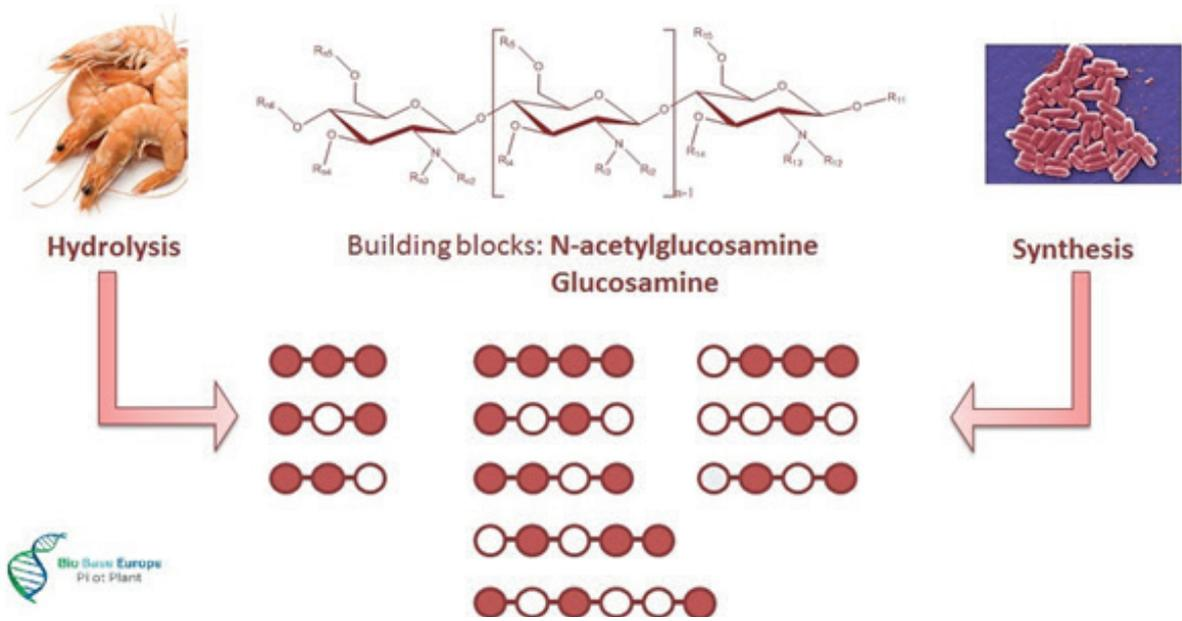
Figure 1: illustration of the two production methods: (left): the traditional chemical process starting from shrimp shell chitin, (right) the new biotechnological approach using glucose and engineered bacteria
